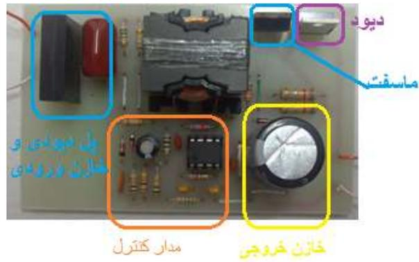
Figure 8. Sample of Boost PFC converter.
