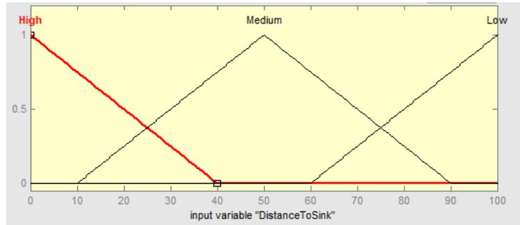
Figure 3. Input membership function, the distance to the plate.
