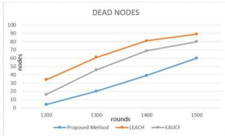
**Figure 9.** The difference of dead nodes number in three LEACH, EAUCF and proposed methods in number of various rounds.
