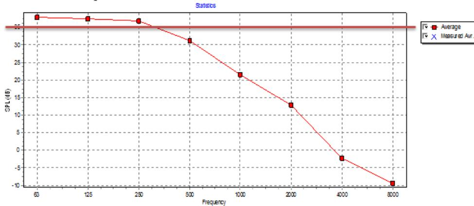
Figure 4. Sound pressure level diagram of LecaBlock.
