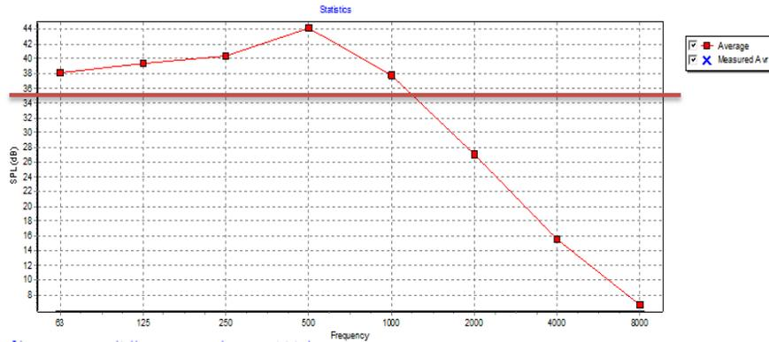
Figure 1. Sound pressure level diagram of Pottery block.
