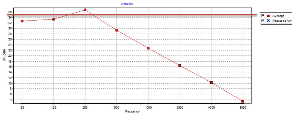
Figure 2. Sound Pressure Level diagram of Hblks block.
