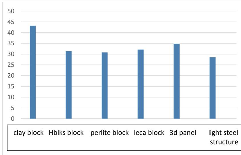
Figure 7. Comparison of modeled audio performance materials.
