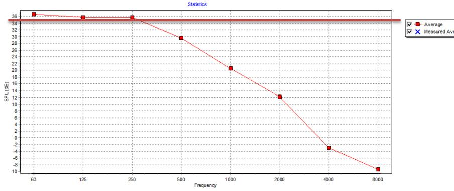
Figure 3. Sound pressurediagram of perliteBlock.
