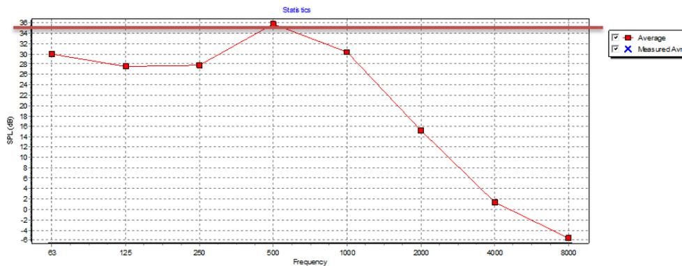
Figure 5. Sound pressure level diagram of 3D panel.
