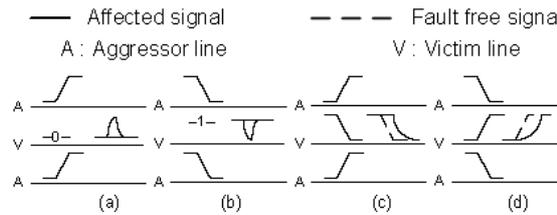
**Figure 1.** Error the hearing: (A) Positive Glitch (b) Negative Glitch (c) Falling Delay Fault (d) Rising Delay fault [13] (A: aggressor line, V: victim line).
