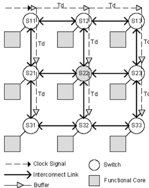
**Figure 4.** Distribution of the clock signal based on the quasi - simultaneously - different skew Between any two adjacent clock against the clock + 1Td Is.
