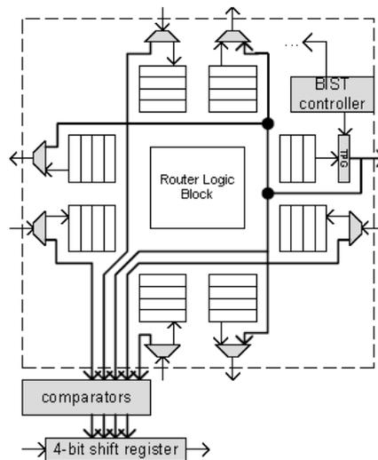
**Figure 3.** Hardware BIST Embedded In A Switched Network With A Mesh Topology Using This Output Buffer.
