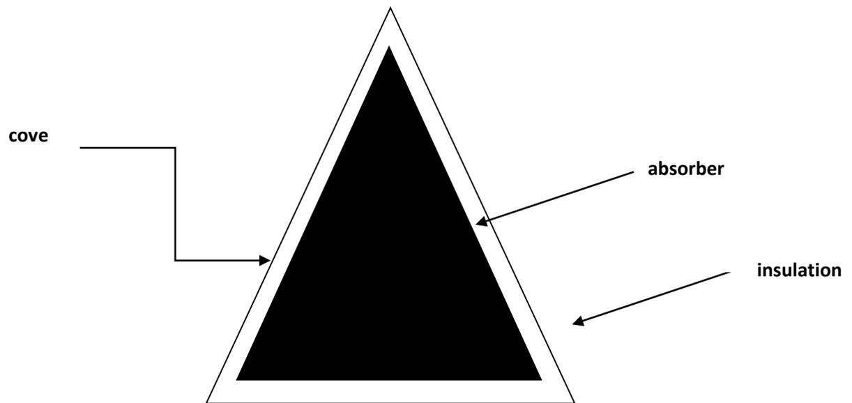
**Figure 1.** The schematic draft of conical solar collector.
