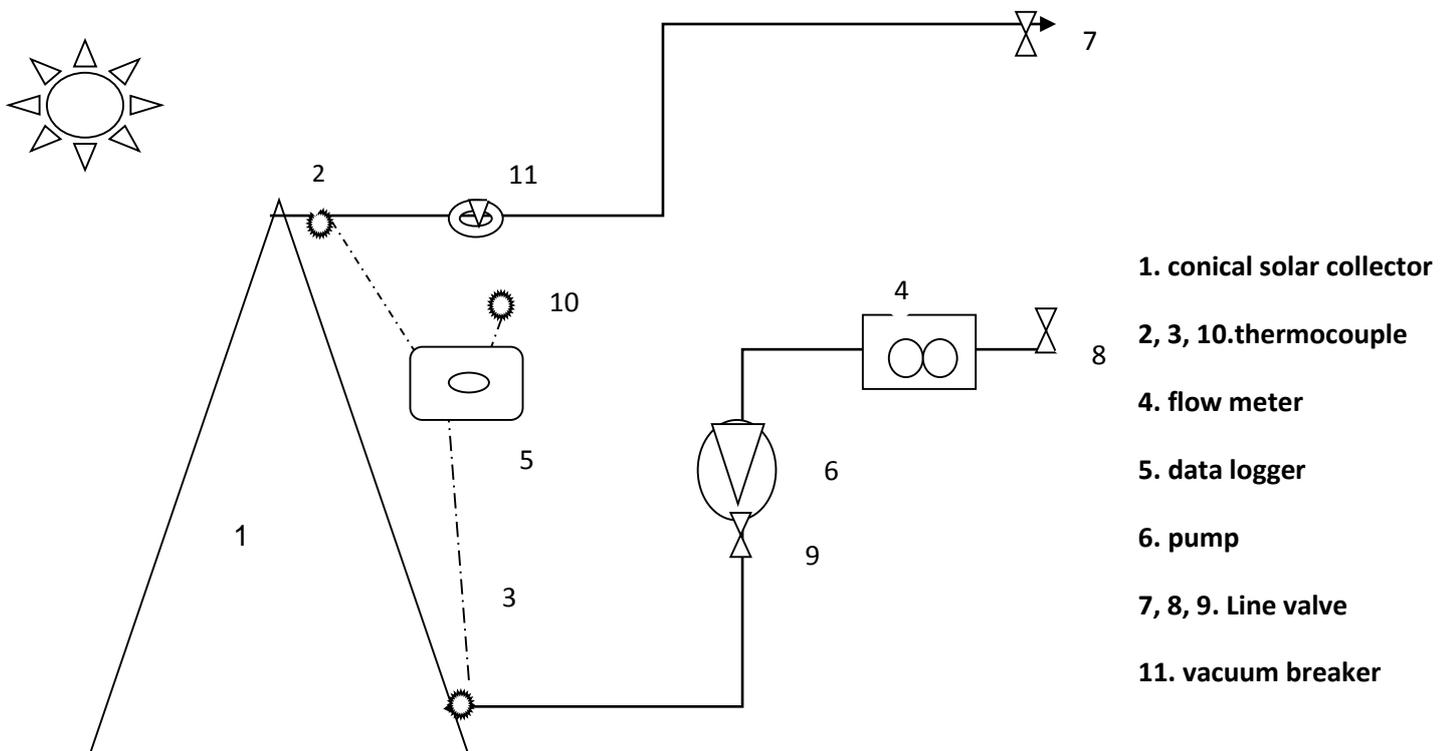
**Figure 4.** The schematic of the experiment.
