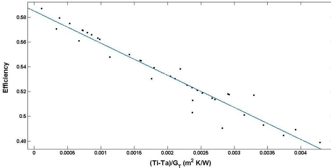
**Figure 6.** The efficiency of solar conical collector.
