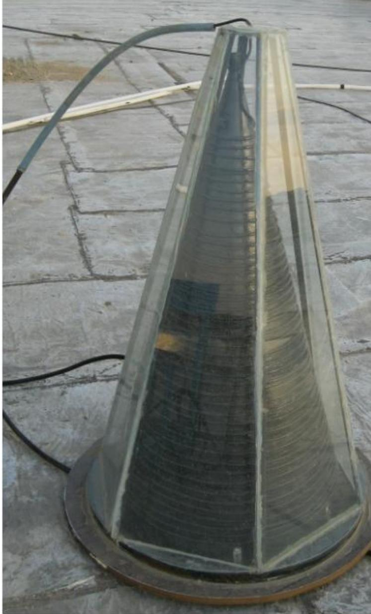
**Figure 3.** The conical solar collector that used in this experiment.
