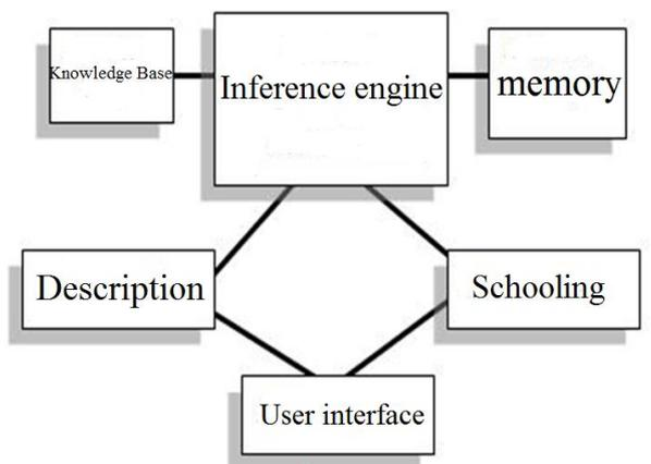
**Figure 1.** The structure of an expert system.
